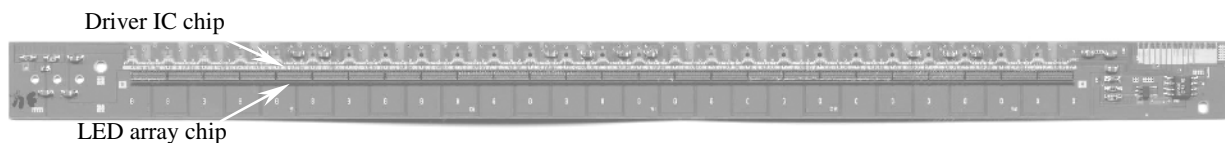
Figure 1. A photograph of the A4-size high-speed high-resolution LED print head.
