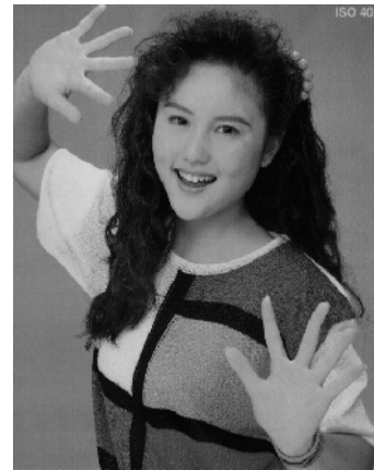
Figure 9. A print sample of the new LED print head. (After reading with an image scanner of 100 dpi.
