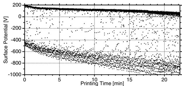
Figure 2. Surface Potential vs. time during printing
