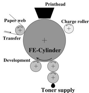
Figure 1. Scheme of the ferroelectric printing system
