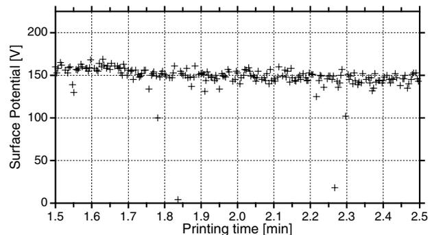
Figure 3. Surface potential in non-imaging areas at the beginning of the printing process
