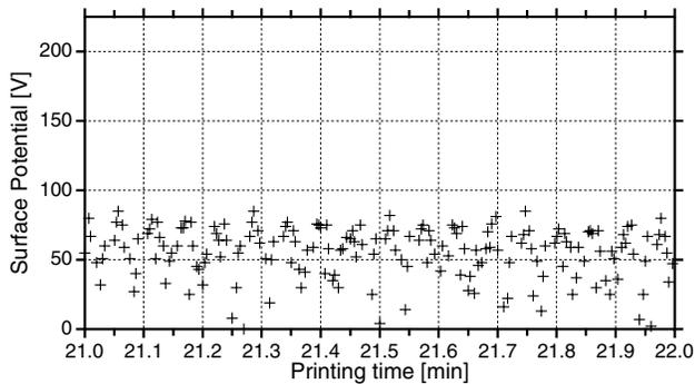
Figure 4. Surface potential in non-imaging areas after 21 min of printing
