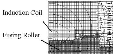
Figure 4. Analysis Model and the Distribution of Magnetic Flux Density
