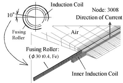
(a) Inner Induction Coil and Fusing Roller
