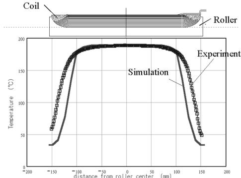
Figure 12. Temperature Distribution (Outer Coil)
