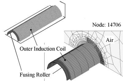
(b) Outer Induction Coil and Fusing Roller
