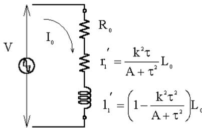
Fig. 3 Equivalent Circuit between the Induction Coil and Fusing Roller
