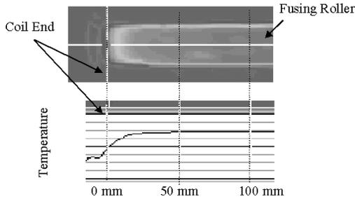
Figure 9. Temperature Distribution (Inner Coil)
