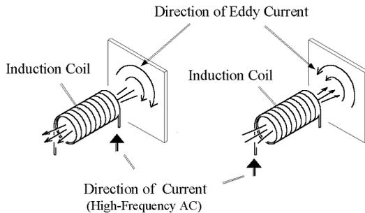
Figure 2. Eddy Current Generated by Induction Coil
