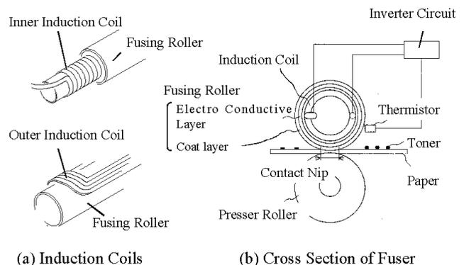
Figure 1. Schematic Diagram of an Induction Heating Fuser
