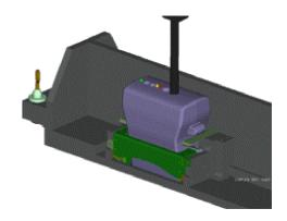
The cartridge can be seen as the basic unit on modular color bar, whereas the color bar on its turn is the basic element in the modular SPICE design. This concept allows us to tailor the digital engine to the customers need; by increasing the number of cartridges on a color bar, Barco can increase the printing width, by increasing the number of color bars, Barco can extend the number of printing colors or the color gamut.
