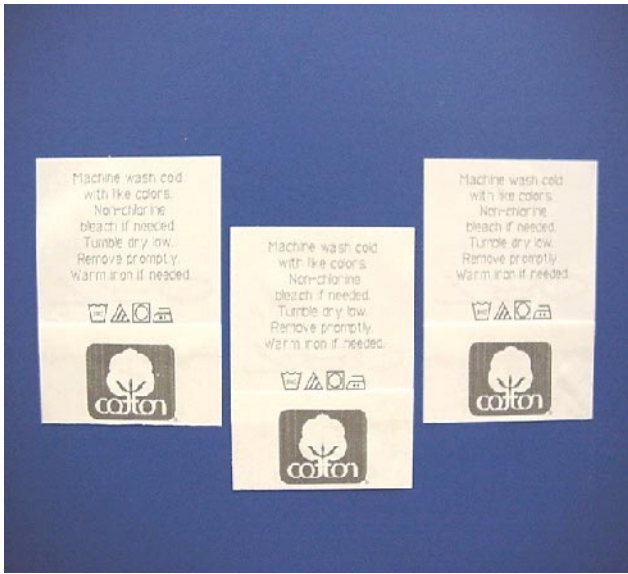
Figure 3. Fabric Label Printed with Liquid DOD Ink Jet. The code is 3/4" x 2".
