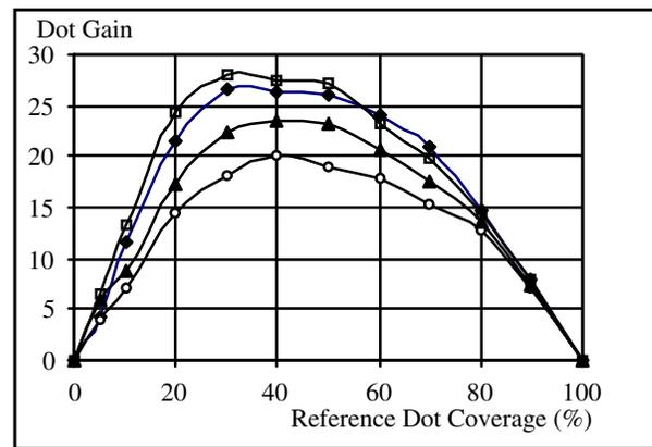
Figure 1. Dot Gain versus Reference coverage
