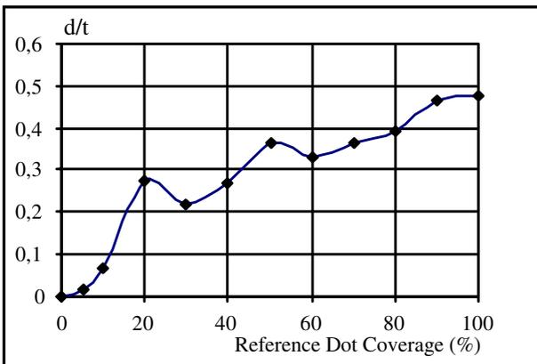
Figure 5. Penetration depth ratio versus dot area (cyan ink)
