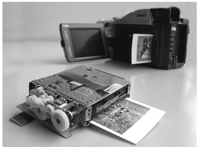
Figure 1. Appearance of PTMTL27 (front) and a camcorder which the unit is built-in (back)
