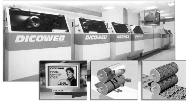
Figure 6. Computer to press / direct imaging system with erasable and re-imageable master (sleeve), (DICOWEB Litho, lab prototype/1995, MAN Roland)
