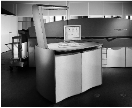
Figure 3. Digital production multicolor sheet-fed printing system with NIP-technology of electrophotography (NexPress 2100: 600dpi, 70 A4 ppm/2100 A3 pph, Heidelberg/Kodak)
