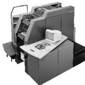
Figure 5. Computer to press/direct imaging system for multicolor waterless offset printing (Quickmaster DI 46-4: 1270/2540 dpi, 333 A4 ppm/10000 A3 pph, Heidelberg)
