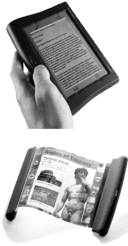
Figure 29. Electronic book (E-book). (a) Rocket eBook/NuvoMedia; (b) Concept study with roll-out screen (Philips)
