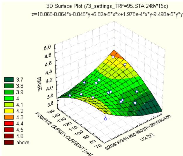
Figure 5. The effect of changing U2 voltage and duplex currents with fixed transfer currents
