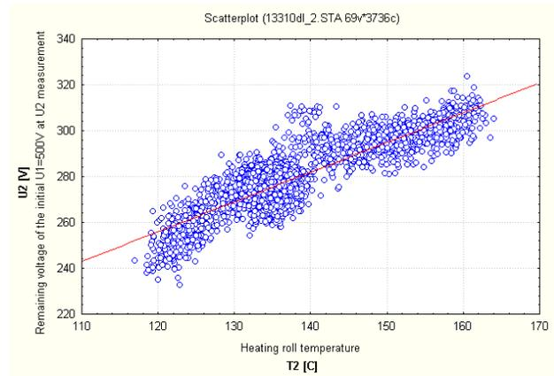
Figure 6. The relation of the voltage relaxation and the intensity of paper drying
