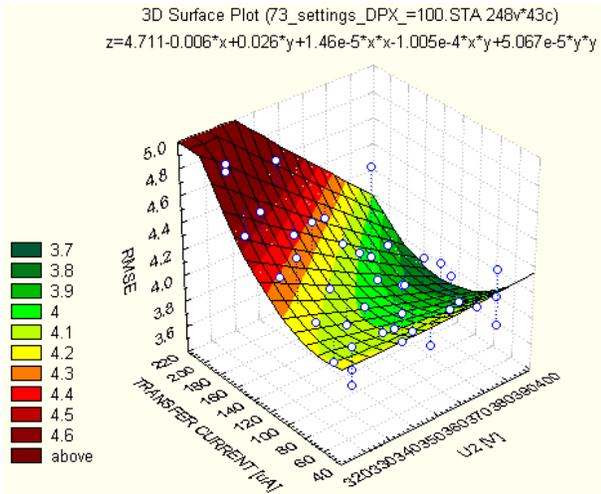
Figure 4. The effect of changing transfer currents and U2 voltage with fixed duplex currents
