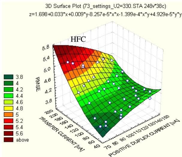
Figure 8. The effect of changing the transfer and duplex currents, moist paper ( $U_2=330$  V)
