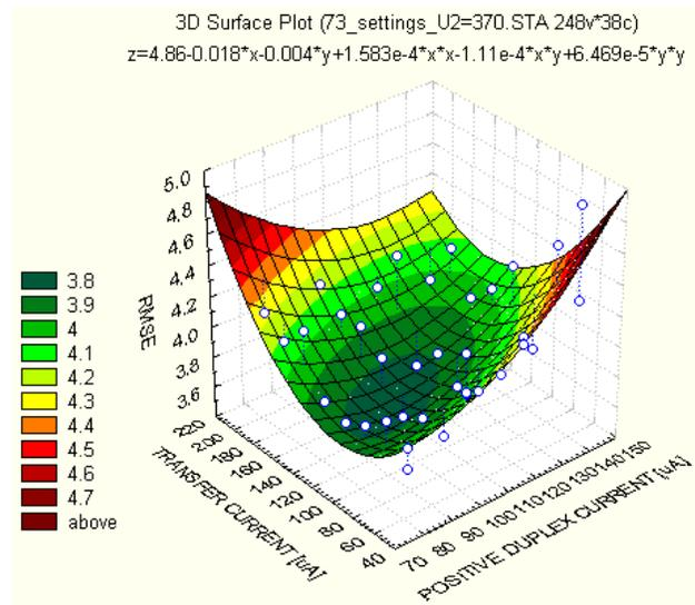
Figure 3. The effect of changing the transfer and duplex currents with fixed U2 voltage
