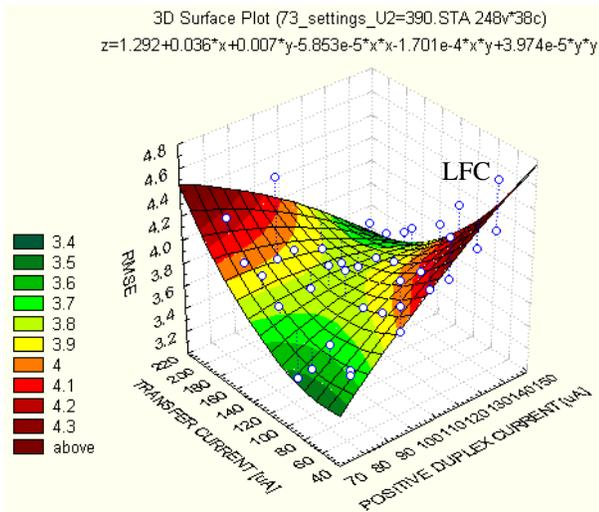
Figure 7. The effect of changing the transfer and duplex currents, dry paper ( $U_2=390$  V)
