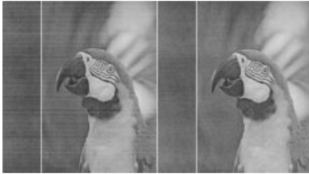
Figure 9: Portion of printed images (3 inch high) scanned at 150 dpi. From the left, 50%-fill test pattern and a halftone image both printed without banding reduction, and the same images printed with banding reduction.
