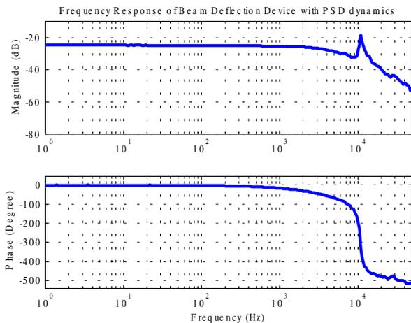
Figure 4: Frequency response of the beam deflection device and PSD circuit combined.
