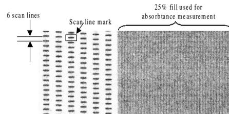
Figure 1: Magnified view of the test pattern used to measure line spacing and absorbance.
