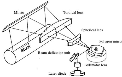
Figure 3: Location of the beam deflection device in the laser pak
