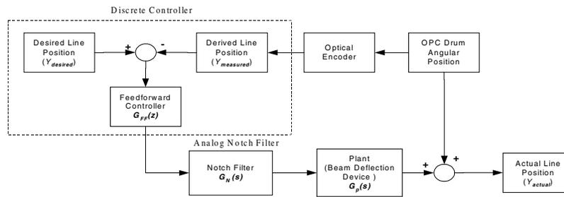
Figure 6: Block diagram of the open loop control system.
