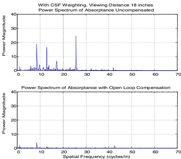
Figure 8: Power spectrum of absorptance variation before (top) and after open loop compensation (bottom).
