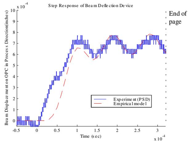
Figure 5: 30 V Step response of the beam deflection device.
