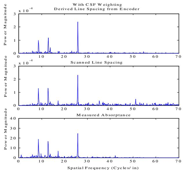
Figure 2: Comparison between the CSF weighted power spectrums of derived line spacing from the encoder, scanned line spacing and absorbance variation.
