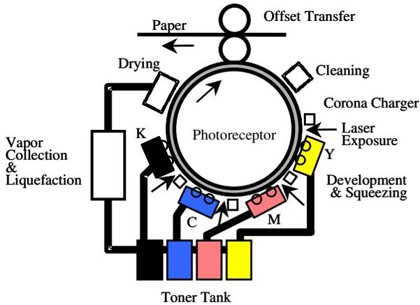
Figure 1. Configuration of liquid toner IOI process
