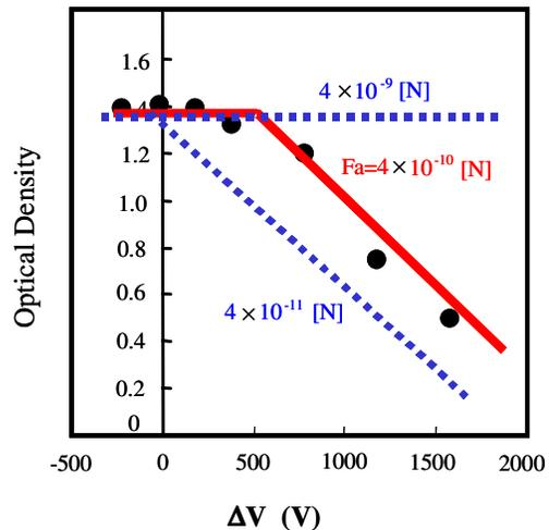
Figure 10. Calculated toner removal characteristics in liquid toner IOI development
