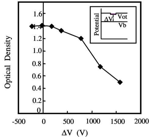
Figure 6. Toner removal in liquid toner IOI development
