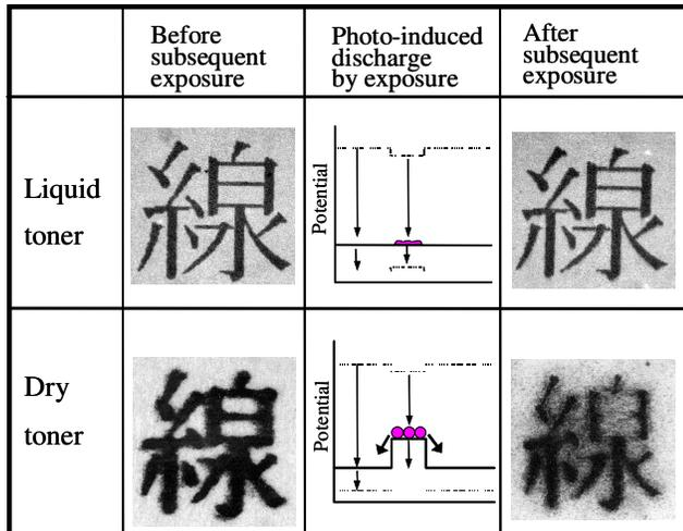
Figure 5. Image comparison between liquid and dry toners before and after subsequent exposure
