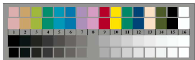
Figure 2. B3&D3: 14 CIE-test colors according to CIE-Publ. 13.3 and B/W + 16 gray steps.
