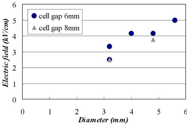
Figure 3. Minimum driving voltage for bi-stable rotation.
