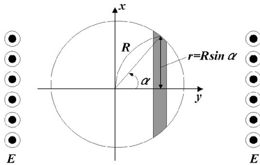
Figure 8. Unit discs within ball: disc parallels electric field.
