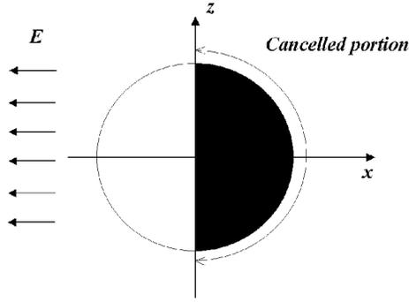
Figure 6. Case 1: Boundary is orthogonal to electric field.
