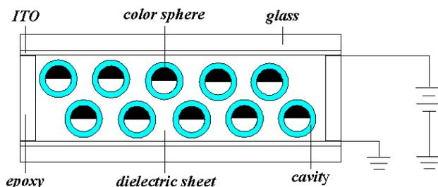
Figure 1. Basic structure of twisting ball display.
