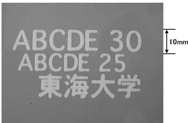
Figure 4. Typical image formed on liquid crystal medium by ion projection (LC type-B, Composition ratio-50/50).
