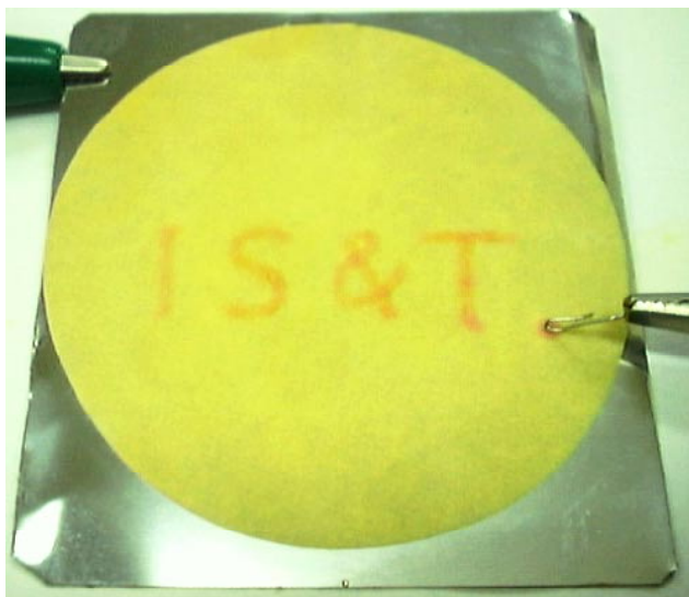
Figure 4. An imaging sample formed by applying DC voltage of 9V.
