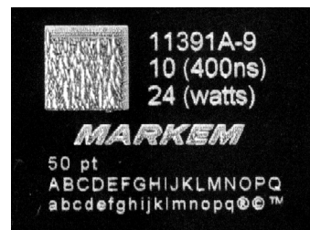
Figure 3. Sample print when carrier film was deformed.
