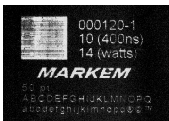
Figure 4. Sample print showing incomplete transfer due to lack of energy conversion.
