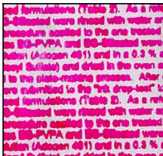
Figure 6: IJ imaged plates; results of A/B interfacial matching: Cationic Ink R2702-1343 on Basic CHB-silicate plate on top (ref. 1a in Table 4) vs. Acidic CHB-PVPA plate on right (ref 10a in Table 4).
