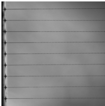
Figure 11. A micrograph of jets ejected from the nozzle array shown in figure 9. The jets are viewed in stroboscopic light when stimulated at a frequency of 1.0 MHz.
