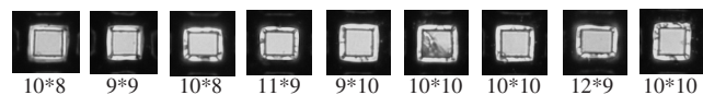
Figure 9. A montage of micrographs of nozzle orifices captured with the aid of an optical microscope. The actual distance between two adjacent nozzles was 500 \mu\text{m} . The white frame surrounding the orifices was due to the illumination light that was reflected in the chamfered edge (sizes in \mu\text{m} ).
