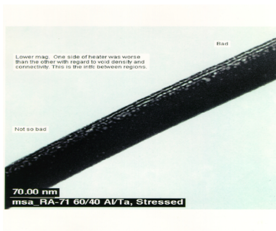
Figure 3. TEM Cross-section of a Failed TaAl Film
