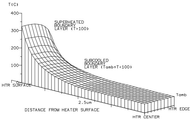
Figure 8: Thermal Boundary Layer in the Ink
