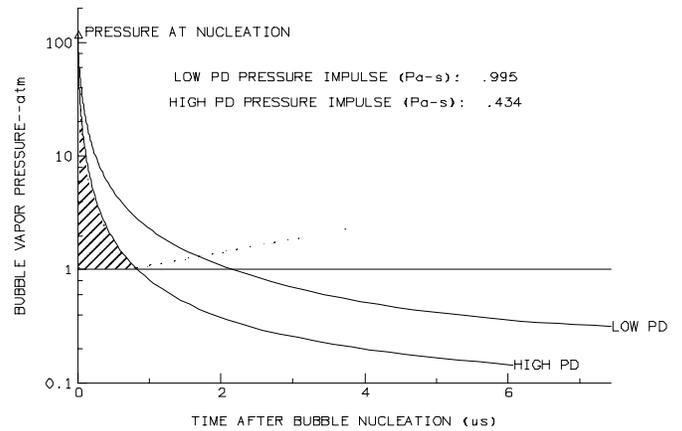
Figure 4: Phase Change Pressure and Power Density
