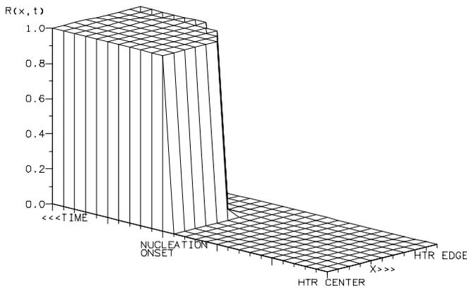
Figure 3: Bubble Reliability Vs Time and Position
