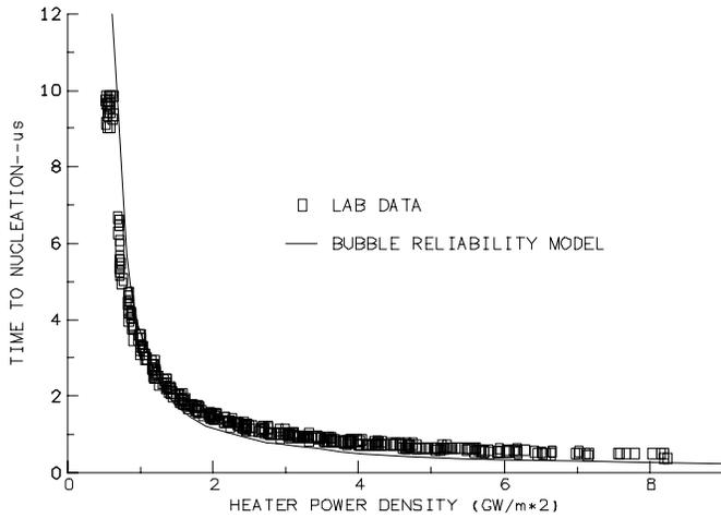
Figure 1: Time to Nucleation Vs Heater Power Density
