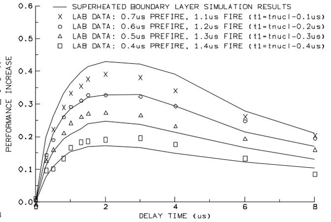
Figure 10: Split Fire Data and Simulations
