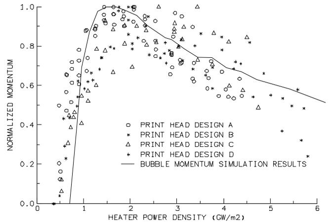
Figure 5: Momentum Vs Heater Power Density
