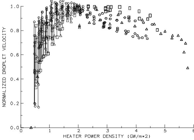
Figure 2: Velocity Response Vs Heater Power Density
