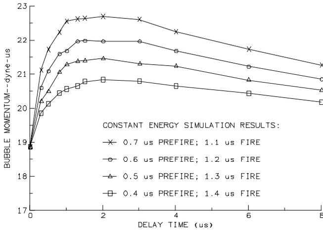
Figure 7: Bubble Momentum and Split Fire Pulsing
