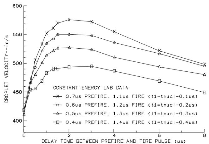
Figure 6: Jet Velocity for Various Split Fire Pulse Trains
