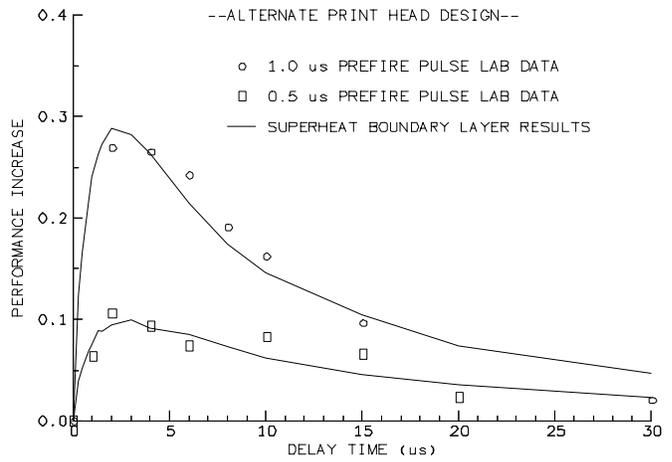
Figure 11: Validation of Hypothesis – Alternate Head Design
