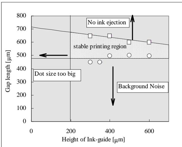
Figure 6. The stable printing region when changing the ink-guide height and the gap between the tip of the ink-guide and the printing material
