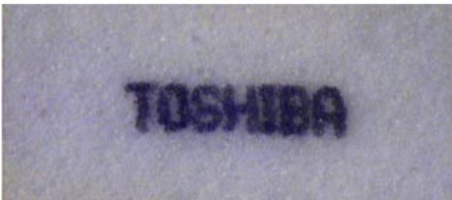
Figure 9. Microstructure letters of 0.1mm size with 5 x 7 dots
