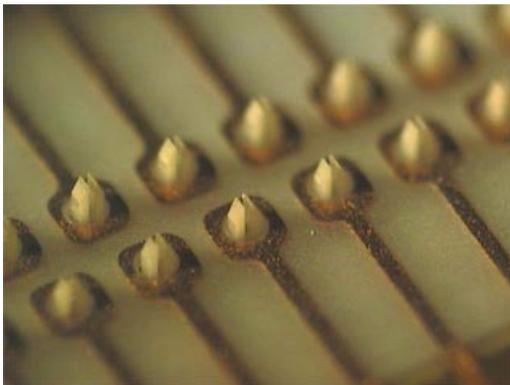
Figure 10. Top view of the control substrate in 4-inch wide printing head and its two rows of apertures
