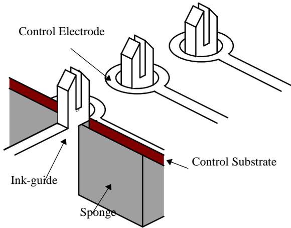
Figure 1. Schematic of the developed printing head
