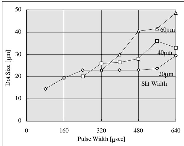
Figure 5. Relationship between diameter of printed dots and the pulse width of signal voltage
