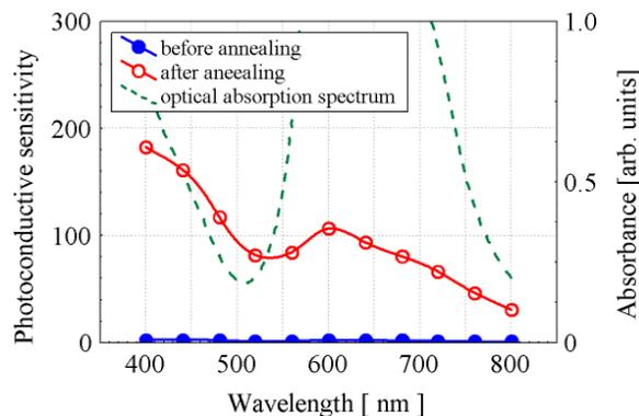
Figure 5. Spectral response of photoconductive sensitivity for C<sub>60</sub> thin film doped with 81mol% of H<sub>2</sub>Pc.
