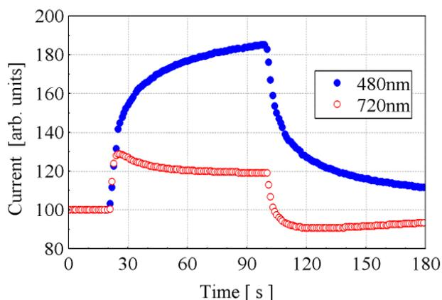
Figure 7. Characteristics of transient photocurrent for  $C_{60}$  thin film doped with 81mol% of  $H_2Pc$  at room temperature.
