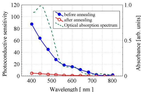
Figure 2. Spectral response of photoconductive sensitivity for C<sub>60</sub> thin film.
