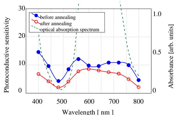
Figure 3. Spectral response of photoconductive sensitivity for H<sub>2</sub>Pc thin film.
