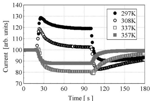
Figure 8. Characteristics of transient photocurrent for  $C_{60}$  thin films doped with 81mol% of  $H_2Pc$  at 720nm at various temperatures.
