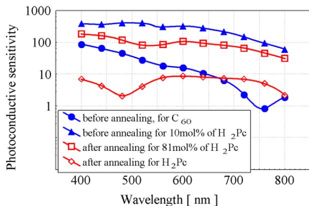
Figure 6. Spectral response of the photoconductive sensitivity for the  $C_{60}$ - $H_2Pc$  coevaporated thin films.
