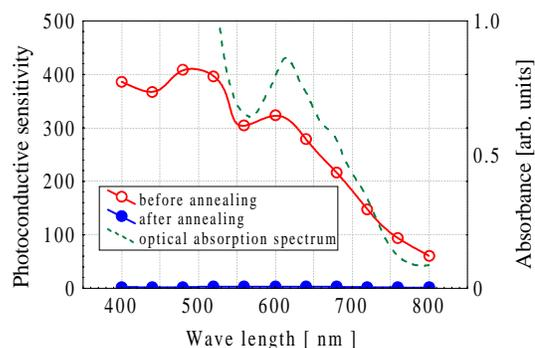
Figure 4. Spectral response of photoconductive sensitivity for C<sub>60</sub> thin film doped with 10mol% of H<sub>2</sub>Pc.
