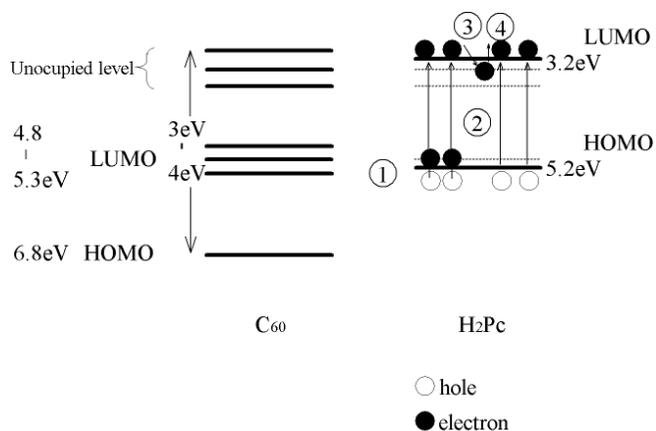
Figure 9. Schematic energy diagram for  $C_{60}$ - $H_2Pc$  coevaporated thin films.
