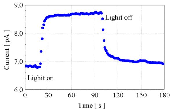
Figure 1. Characteristic of transient photocurrent for  $C_{60}$  thin film at 480nm.
