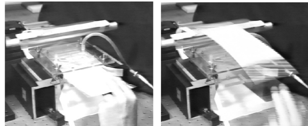
Figure 4. Photographs of small paper mover module with 2-sided forward acting jets, followed by plastic 180° reversion guide. Note that paper flies stably through "open air".
