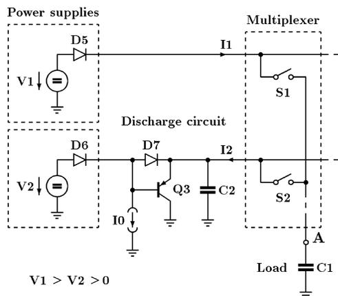
Figure 5. Schematic of the discharge circuit (positive voltages)
