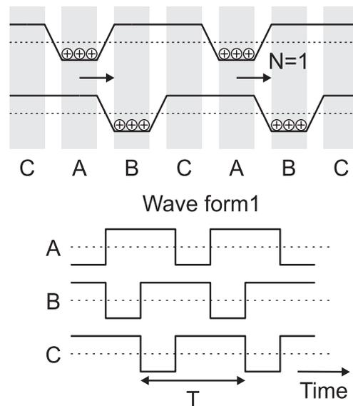
Figure 1. Charged particle transport
