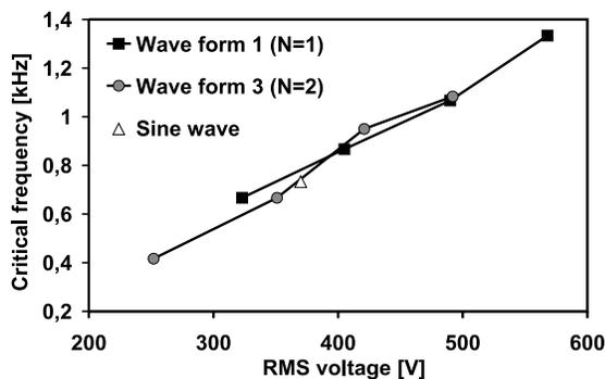
Figure 6. Critical frequency as a function of the RMS voltage applied between adjacent electrodes
