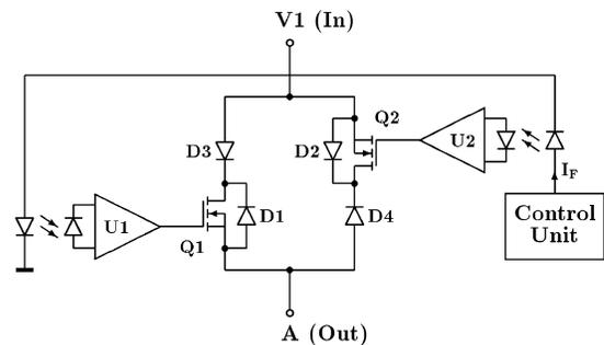
Figure 4. Schematic of a switch (Example:  $S1$ )
