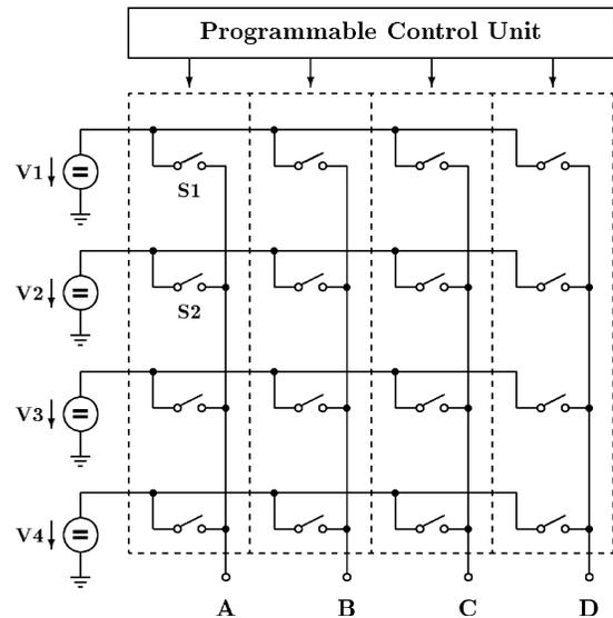
Figure 3. 4-channel multiplexer consisting of 16 switches
