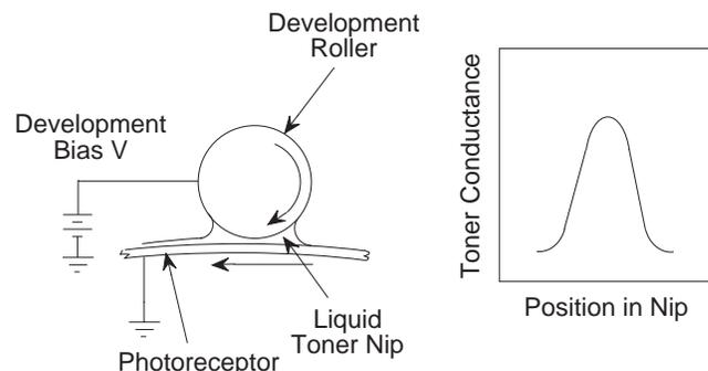
Figure 2. Liquid Toner Nip (Inverted) and Conductance Profile
