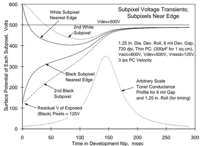
Figure 8. Voltage Transients for Subpixels Near Edge; Large Black Areas Separated by One White Pixel
