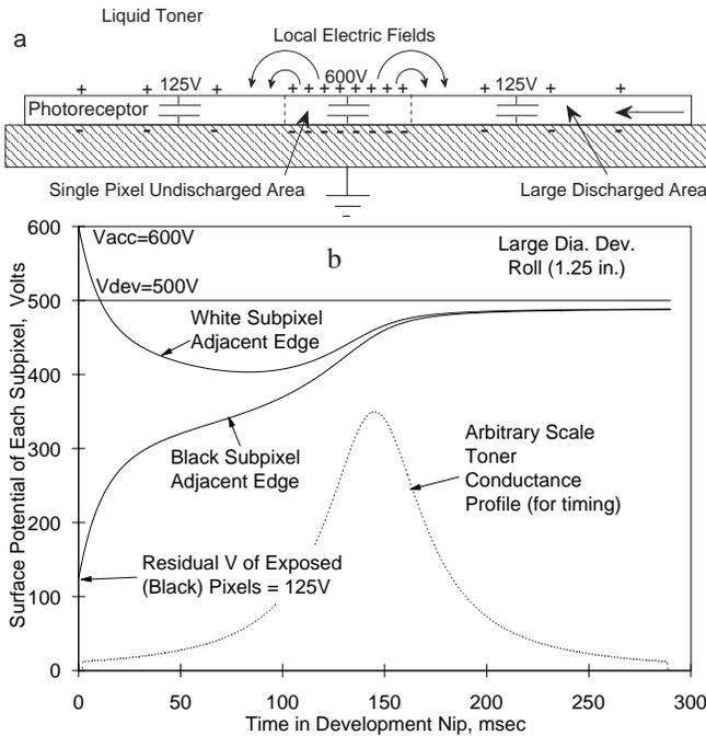
Figure 5. Voltage Transients; Pixel-Pixel Cross Talk Through Liquid Toner
