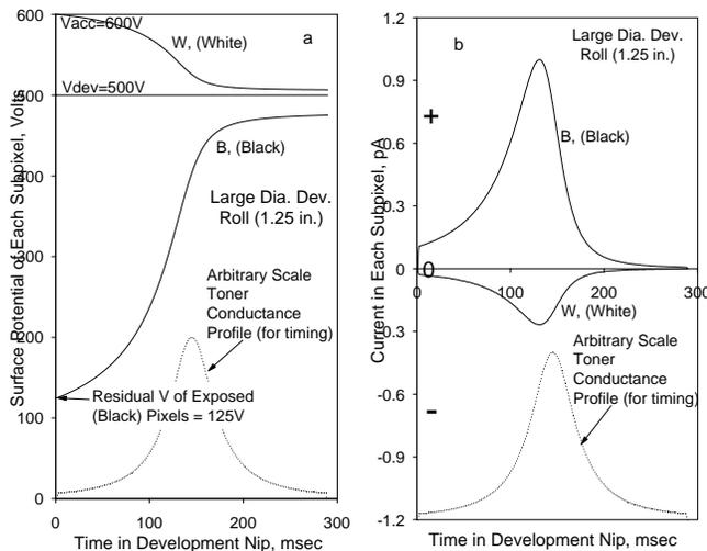
Figure 4. Typical Voltage and Current Transients for a White and Black Pixel; Non-Cross Talk Case
