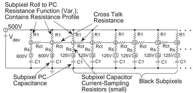
Figure 7. Simplified Analog Circuit Model
