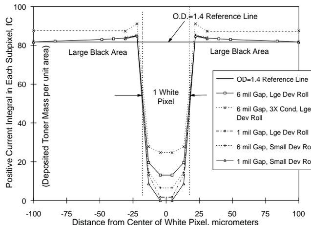
Figure 10. Deposited Toner Profiles Across Single White Pixel
