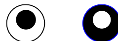
Figure 1. Cross Sectional view of the two types of fibers used for conductive brush cleaning. The black represents the conductive polymer.
