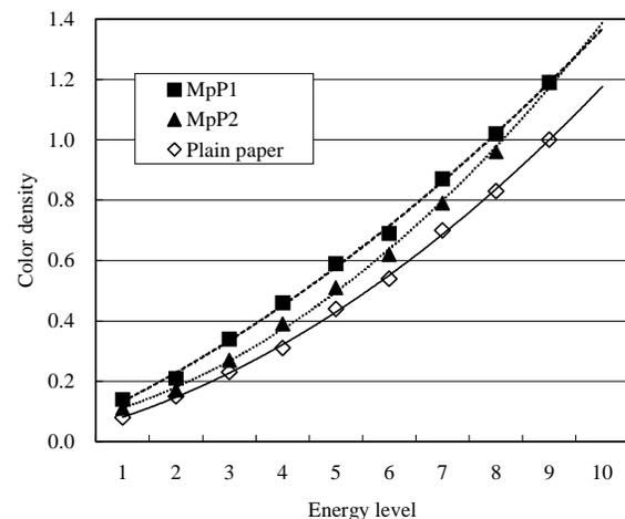
Figure 2. Color (cyan) densities of the micro-porous paper sheets as a function of energy level
