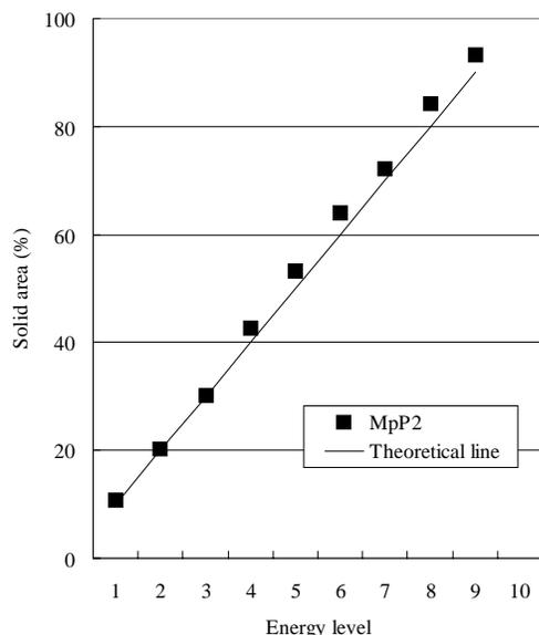
Figure 3. Continuous tone reproducibility (magenta) of the micro-porous paper sheet (MpP2) as a function of energy level
