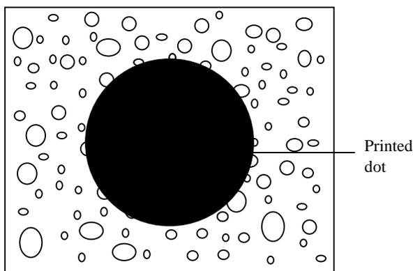
Figure 1. Surface view of a micro-porous layer for use in thermal wax transfer printing
