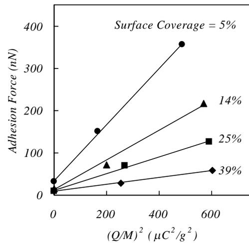
Figure 5. Dependence of the average adhesion force on the square of toner charge to mass ratio,  $(Q/M)^2$ .
