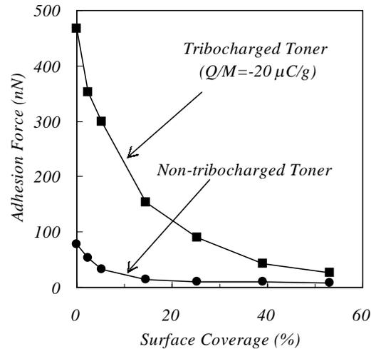
Figure 7. Relationship between the average adhesion force and the toner surface coverage for the non-tribocharged toner and the tribocharged toner.
