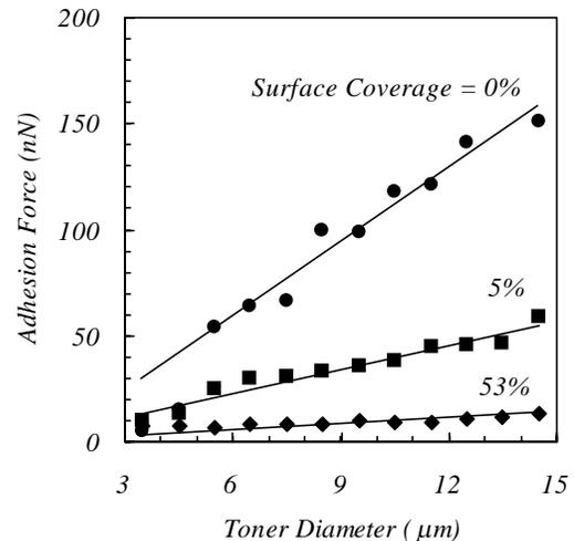
Figure 2. Size dependence of the adhesion force for the non-tribocharged toner.
