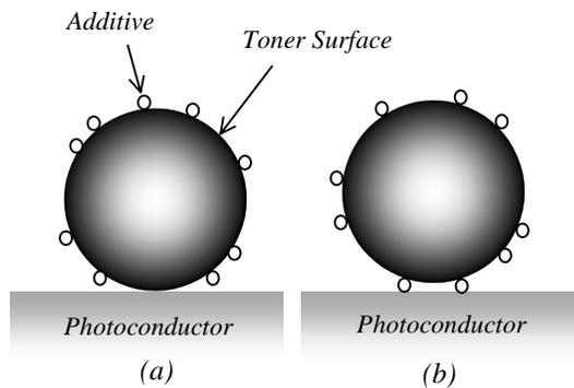
Figure 4. The contact models between a toner particle with additives and a photoconductor; (a) toner surface contacts a photoconductor, (b) additives contact a photoconductor
