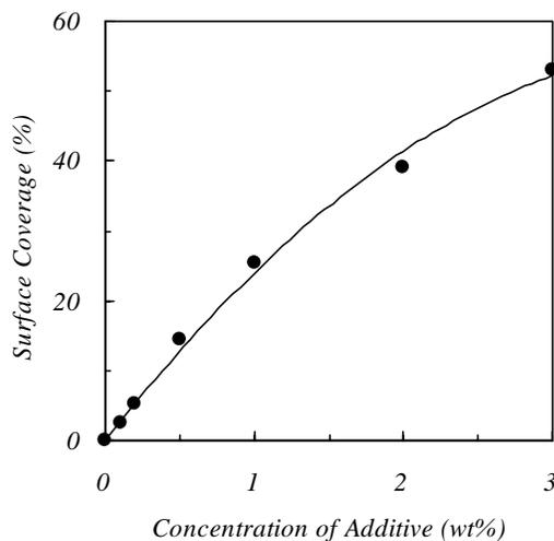
Figure 1. Relationship between the toner surface coverage by additive and the concentration of additive.
