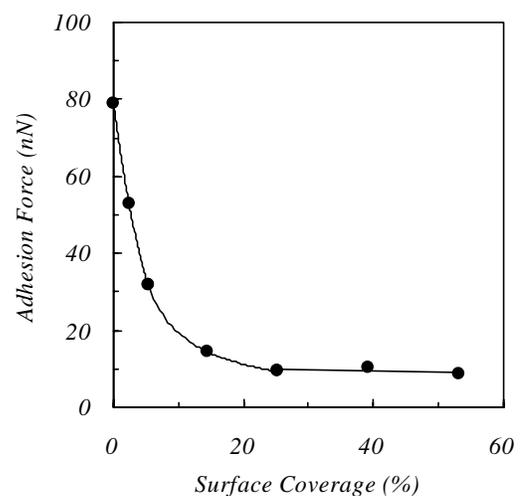
Figure 3. Relationship between the average adhesion force and the toner surface coverage for the non-tribocharged toner.
