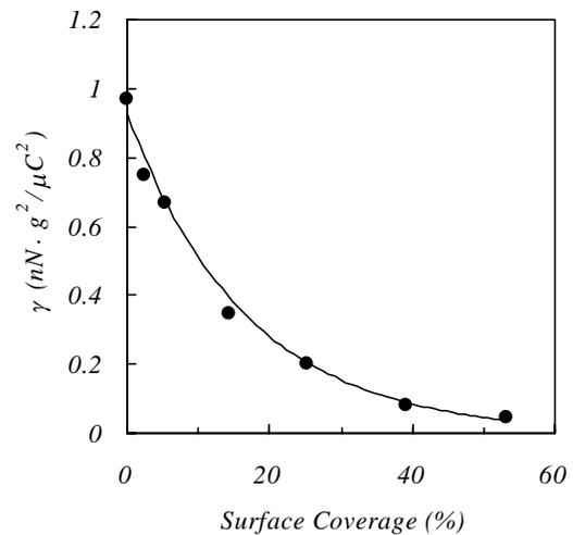
Figure 6. Slope between the average adhesion force and  $(Q/M)^2$ ,  $\gamma$  plotted against the toner surface coverage.
