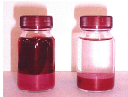
Figure 6. Desorption test from COP; left:neutral (non cationized); right : COP (cationized)
