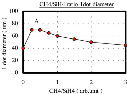
Figure 6. The relation with CH4/SiH4 and 1 dot diameter
