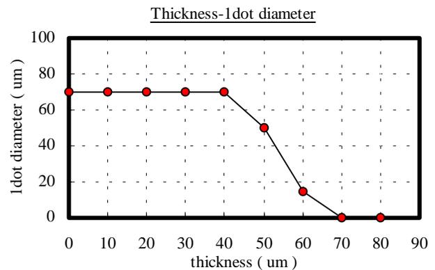
Figure 9. The relation with thickness and diameter (after interface condition changed)
