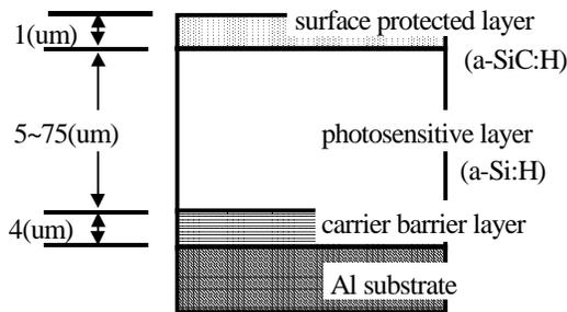
Figure 3. The structure of a-Si photoreceptor
