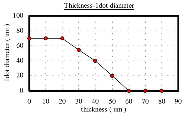
Figure 4. The relation with thickness and 1-dot diameter (before interface condition changed)
