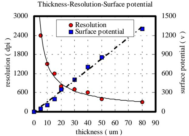
Figure 11. The relation to thickness-resolution-surface potential
