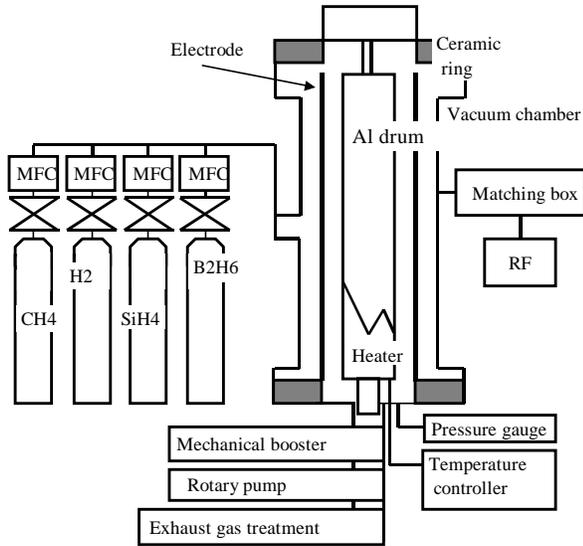
Figure 2. The schematics of diagram of plasma CVD equipment
