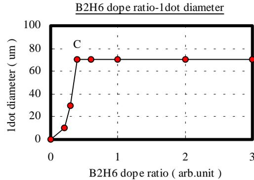
Figure 8. The relation with B2H6 dope ratio and 1 dot diameter
