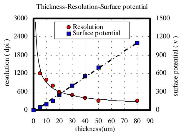
Figure 1. The relation of thickness-resolution-surface potential (before improvement)
