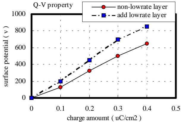
Figure 10. Q-V property (the effect of low rate layer)
