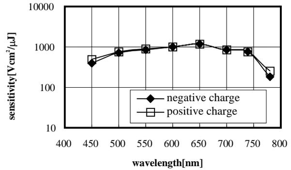
Figure 5. Spectral sensitivity characteristics of negative and positive charge drums to reduce surface potential from 500V to 50V.
