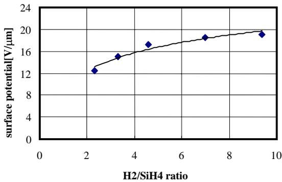
Figure 3. Relation between H<sub>2</sub>/SiH<sub>4</sub> ratio in photosensitive layer and surface potential normalized by film thickness when charge amount is 0.3 μC/cm<sup>2</sup>.
