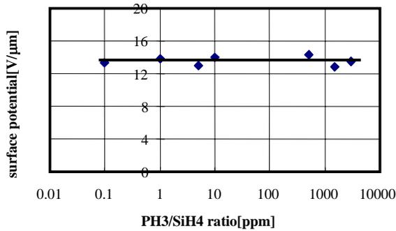
Figure 2. Relation between PH<sub>3</sub>/SiH<sub>4</sub> ratio in carrier blocking layer and surface potential normalized by film thickness when charge amount Q is 0.3 μC/cm<sup>2</sup>.
