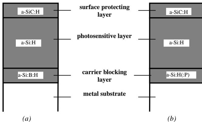
Figure 1. Layer constructions of (a) positive charge a-Si drum and (b) negative charge a-Si drum
