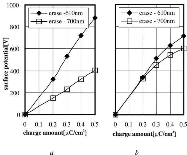
Figure 8. Difference in Q-V characteristics when wavelength of erase lamp is varied for (a) positive charge and (b) negative charge drum.
