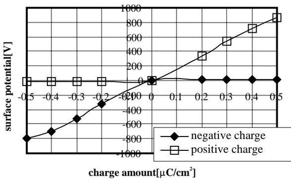
Figure 4. Q-V characteristics of negative and positive charge drums.
