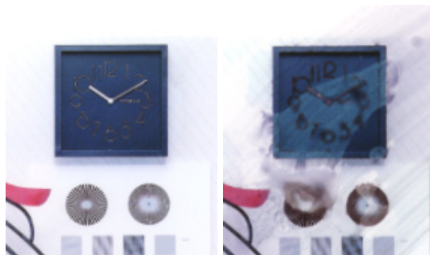
Figure 7. Water resistance testing of QP paper (left) and a swelling paper (right)
