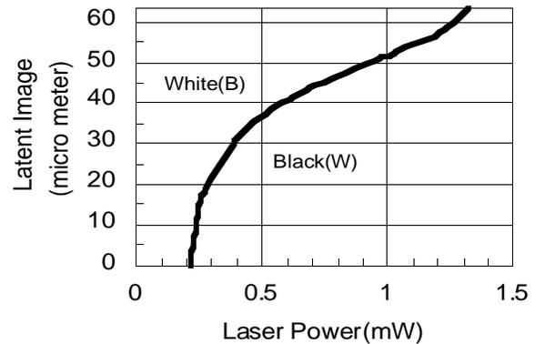
Figure 5. Black and White line width of 1-On/1-Off repeated lines on the reversal development. Parenthesis shows the case of the normal development.
