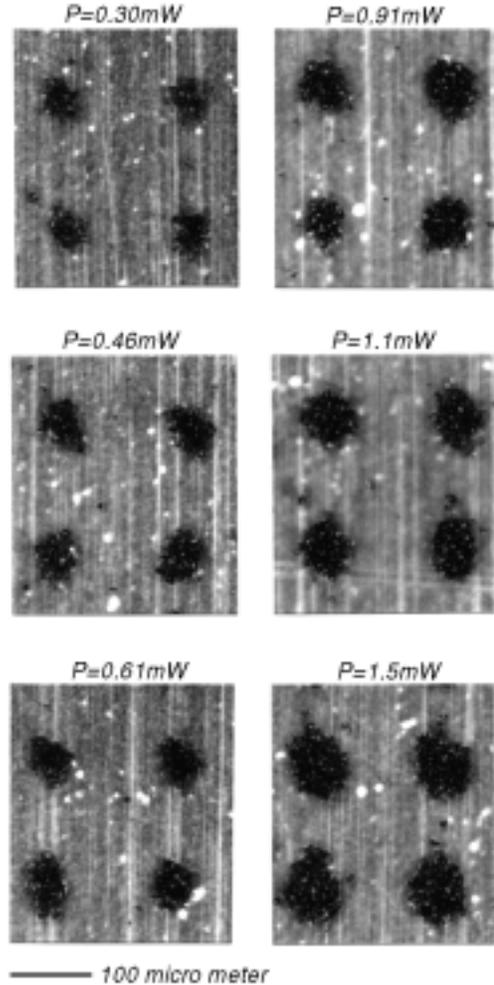
Figure 2. Toner Image of one dot printing on photoreceptor. Horizontal direction is scanning one of laser beam. P is the value of laser power at the photoreceptor.
