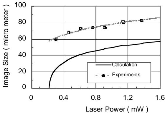
Figure 3. Comparison between calculation and experiments of one dot image size.
