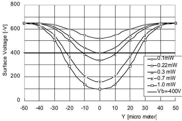
Figure 1. Surface voltage distribution. The values of insert are input power (P) on the photoreceptor at the position y=0 and the biased voltage (Vb) of development.
