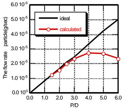
Figure 5. Relation between the flow rate of particle and the rate of the screw pitch to the screw diameter ( $P/D$ ).
