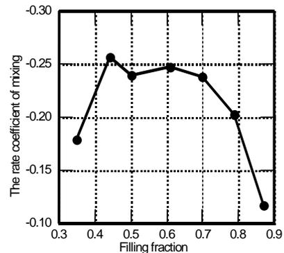
Figure 4. Relation between the rate coefficient of mixing and filling fraction.
