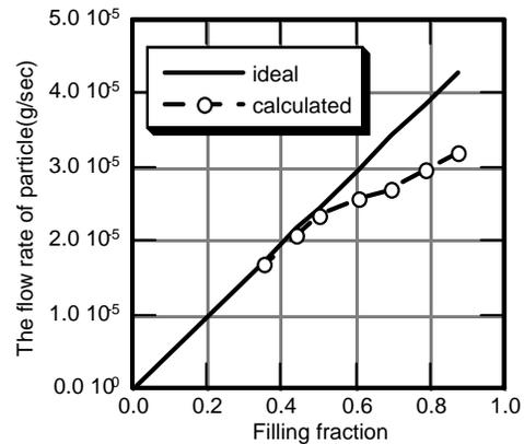
Figure 3. Relation between the flow rate of particle and filling fraction.
