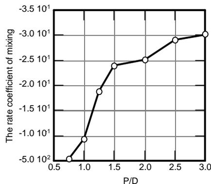
Figure 6. Relation between the rate coefficient of mixing and the rate of the screw pitch to the screw diameter ( $P/D$ ).
