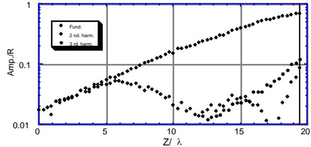
Figure 4. Multimode stimulation for  $k=0.69$ . Growth of fundamental and harmonics
