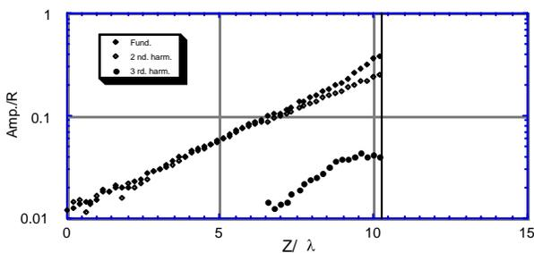
Figure 6. Multimode stimulation for  $k=0.45$  and  $\varphi=0^\circ$ . Growth of fundamental and harmonics
