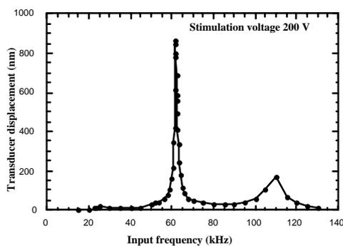
Figure 2. Transducer displacement versus frequency
