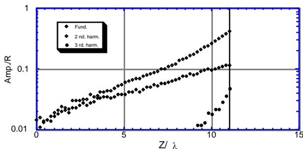
Figure 7. Multimode stimulation for  $k=0.45$  and  $\varphi=180^\circ$ . Growth of fundamental and harmonics
