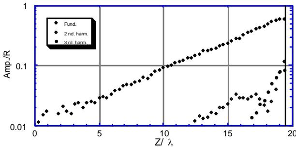
Figure 3. Normalized amplitudes of fundamental and harmonics for  $k=0.69$  and sinusoidal stimulation signal
