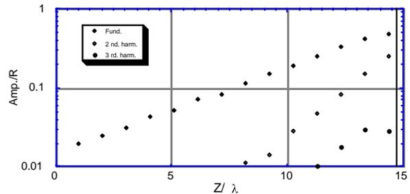
Figure 5. Normalized amplitudes of fundamental and harmonics for  $k=0.45$  and sinusoidal stimulation signal
