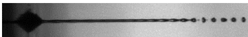
Figure 6. A jet ejected from a square orifice changes to cylindrical shape after a few droplet diameters. This can be seen as the waves on the jet close to the nozzle. The waves that cause break-up of the jet grow as the jet travels and are not visible until close to the droplet formation point.
