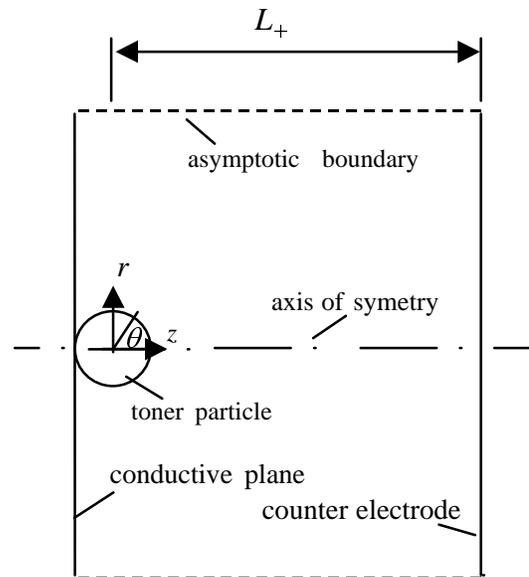
Figure 1. Definition sketch of a toner particle resting on one of the electrodes in a parallel-plate capacitor
