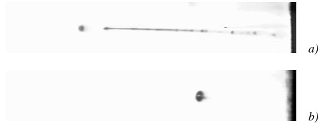
Figure 1. The jets of the standard ink (a) and polyacrylamide solution of concentration of 100 p.p.m. and molecular mass of 2,000,000 (b). Jet motion is from right to left. Longitudinal frame size corresponds to 2 mm. The flight time is 140 \mu s.
