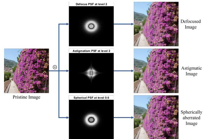
**Figure 1.** An illustration summarizing the aberration simulation process. The PSFs are generated in ISETcam and then convolved with the reference image to obtain the aberrant images
