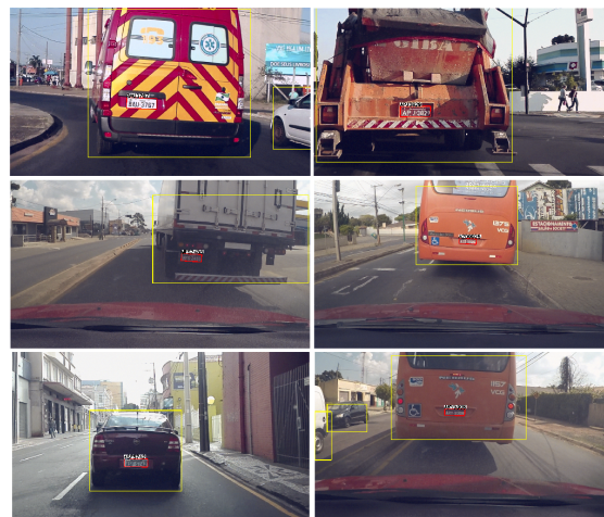
Figure 7. Examples of vehicles for which recognition became successful after introducing read noise.
