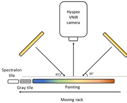
Figure 2. The scheme of the imaging setup.
