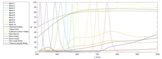
**Figure 8.** Simulated sensitivities of the Visible-only camera and the spectra of spectral library members.
