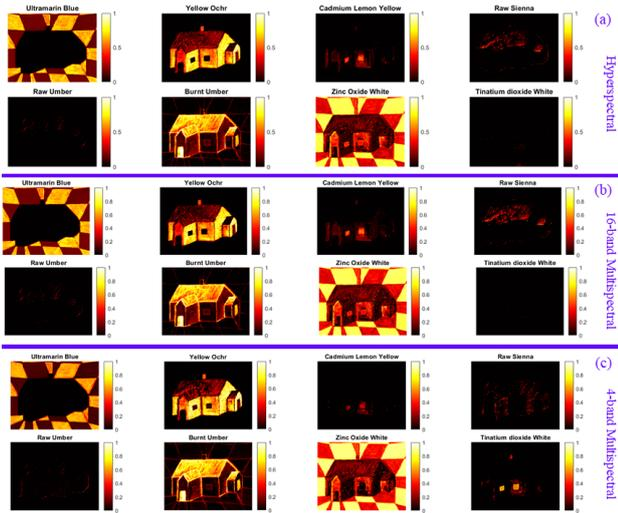
**Figure 6.** Comparison of the pigment maps obtained from: a) Hyperspectral camera, b) 16-band Multispectral camera, c) 4-band Multispectral camera
