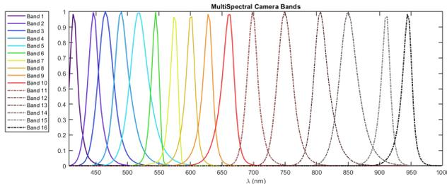
Figure 3. The Spectral sensitivity of the simulated multispectral camera.
