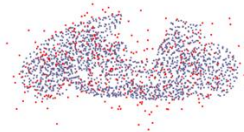
Figure 5: Corrupted MVP point cloud to be filtered using the minimum nearest neighbor average distance approach
