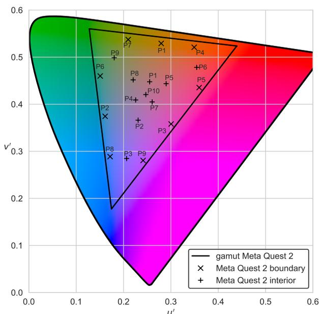
Figure 1: The chromaticity gamut of the Meta Quest 2 HMD is shown as a black triangle. The boundary points are annotated as 'x' markers and the interior points as '+' markers. Note that the colours on the diagram are solely for reference and may not accurately reflect specific colours.
