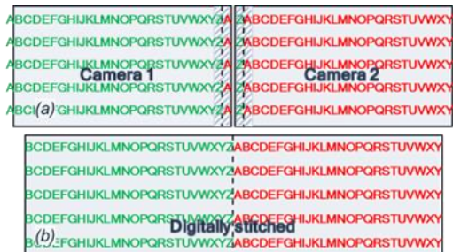
Figure 7. (a) Images see by the TPC two cameras with overlapping areas (shaded). (b) A stitched TPC image
