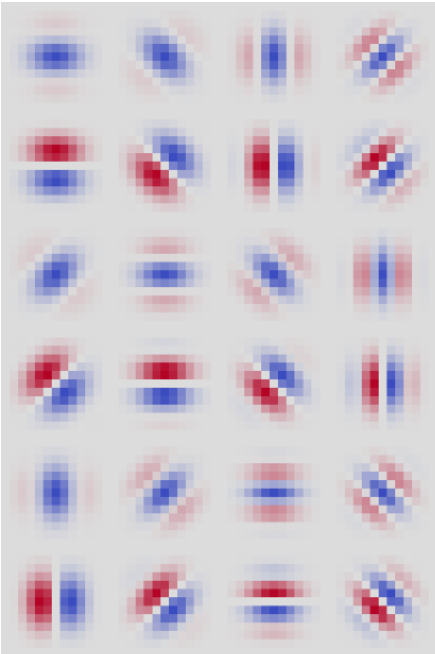
Figure 1. The original bank of Gabor filters before refactoring.
