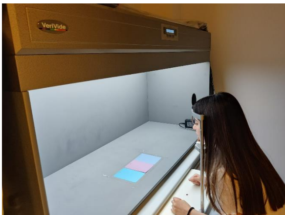
Figure 3. Setup of the visual experiment conducted to obtain a visual graininess scale.
