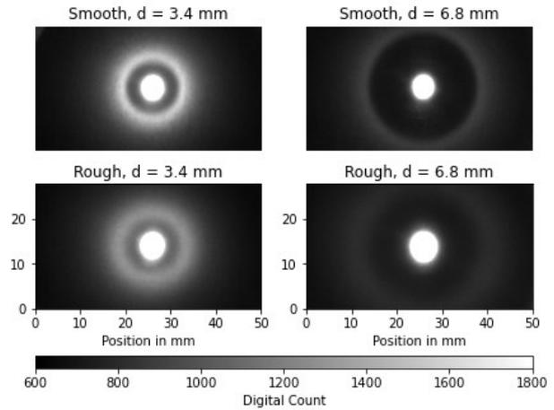
Figure 6. Pictures of the halo induced by a smooth and a rough interface with air for two different coating thicknesses.
