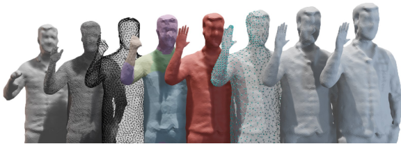
Figure 4. Mesh tracking and registration is typically applied for efficient representation and to enable editing of VV [6].
