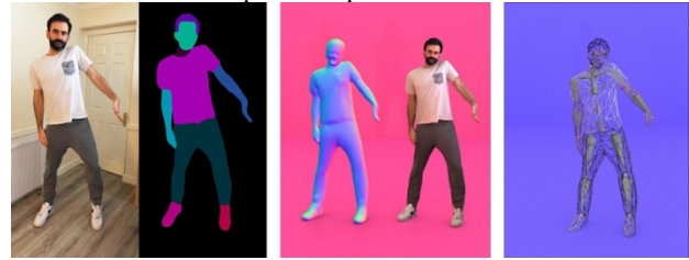
Figure 5. Different steps in the Volograms AI pipeline that use deep learning. Left: input image and semantic segmentation. Centre: volumetric reconstruction without and with texture. Right: underlying 3D skeleton.
