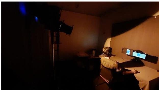
**Figure 1:** An observer performing the experiment with 50 lux illuminance and 50 cd/m<sup>2</sup> display luminances.
